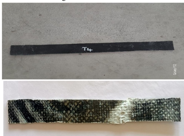
Fig-3.2 After tensile test
