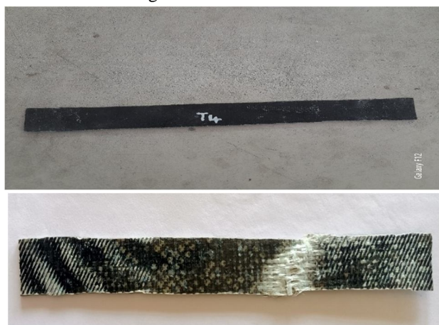
Fig-3.2 After tensile test
