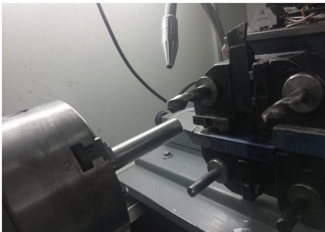
Fig. 11 Machining operation with tungsten carbide tool at both lubricant
