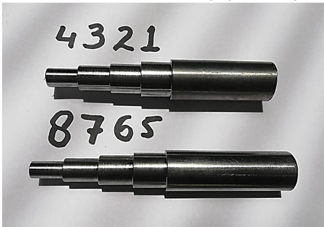
Fig. 16 Workpiece of titanium alloy (Ti-6Al-4V) after tuning
