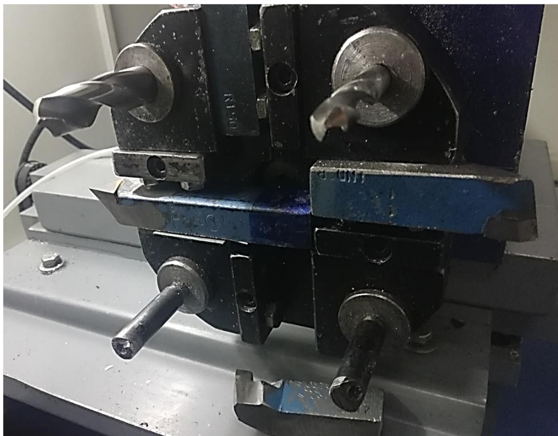
Fig. 9 Tungsten carbide tool with tool holder
