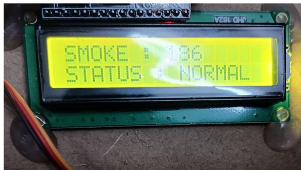
FIG.8.Message display after gas leakage in LCD
