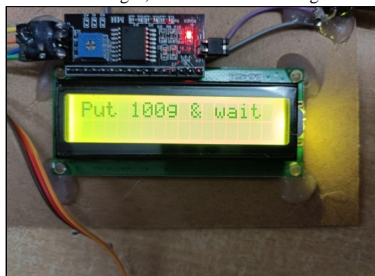
FIG.5. Output on the LCD display before putting load on the Load Cell
