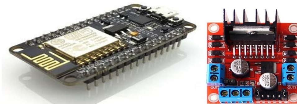
Fig. 2 Diagram of NodeMCU board and L298N motor driver.
