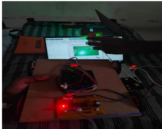
Fig 3. Green signal is captured by the camera and the vehicle starts moving again
