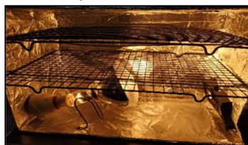
Figure 2 Food Dehydrator Developed by us at GIFT Campus
