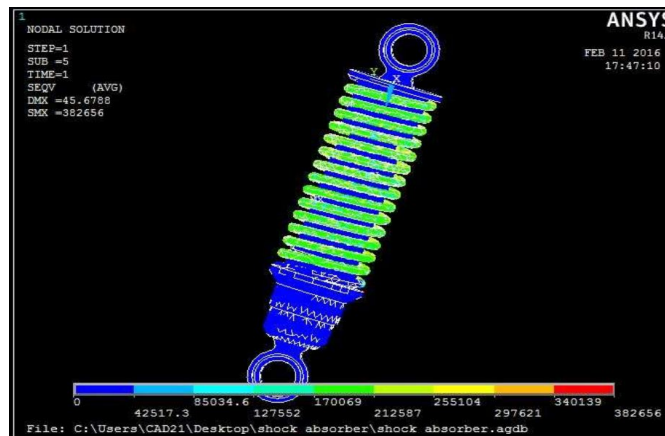
Fig -10: Von Mises Stress for Steel spring
