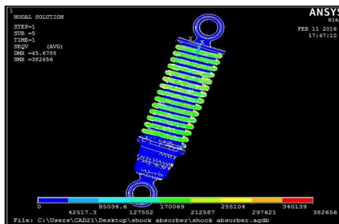
Fig -10: Von Mises Stress for Steel spring
