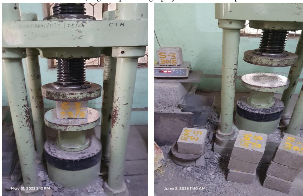
Fig. 2 Compression testing machine with geopolymer concrete samples
