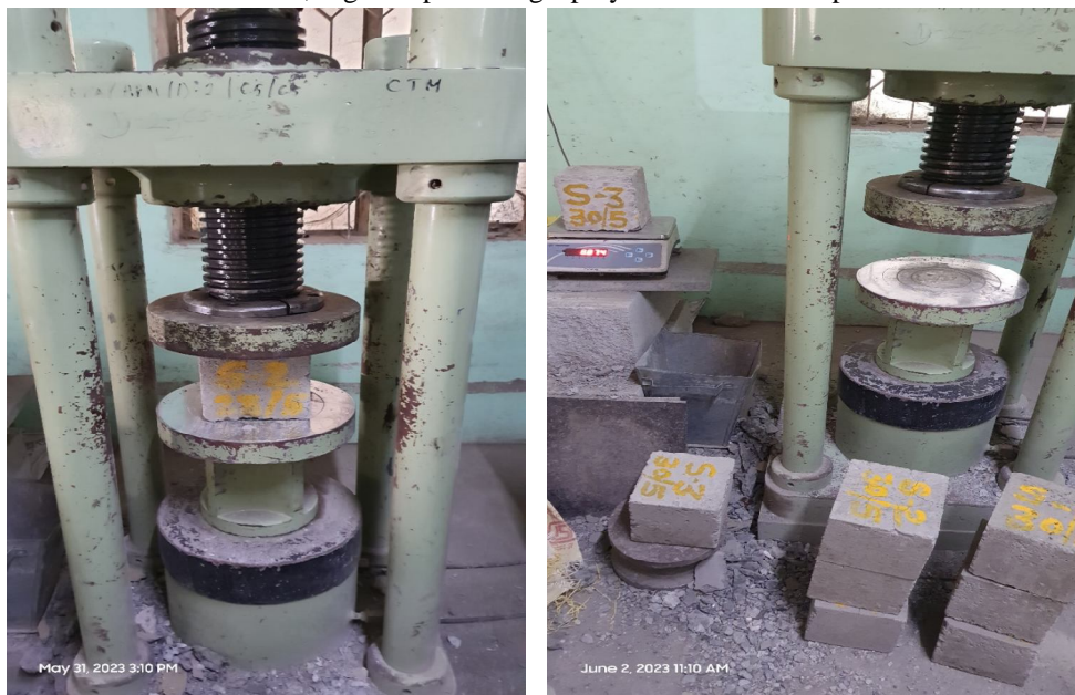
Fig. 2 Compression testing machine with geopolymer concrete samples
