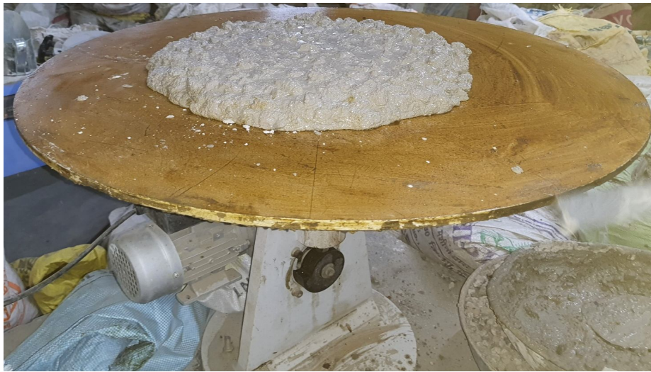
Fig. 1 Flow table apparatus with fresh geopolymer concrete mix.
