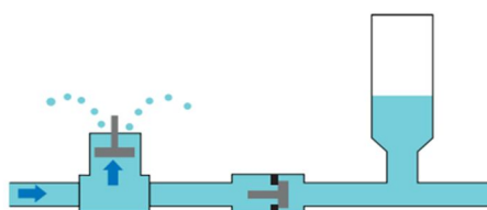
FIGURE 18: The automatic HRP working cycle.
