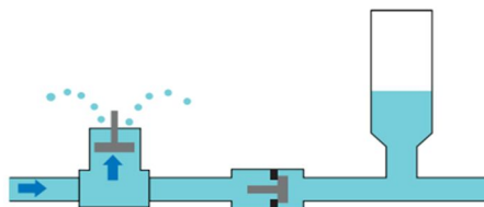
FIGURE 18: The automatic HRP working cycle.
