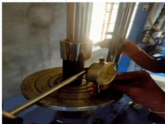
Fig.2. Normal Soil Specimen Undergoing UCS Test
