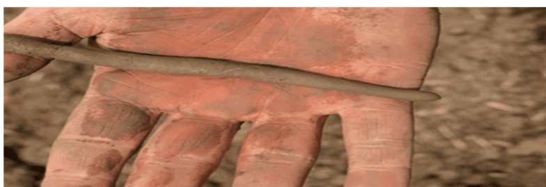
Fig.8 Plastic limit Soil Thread
