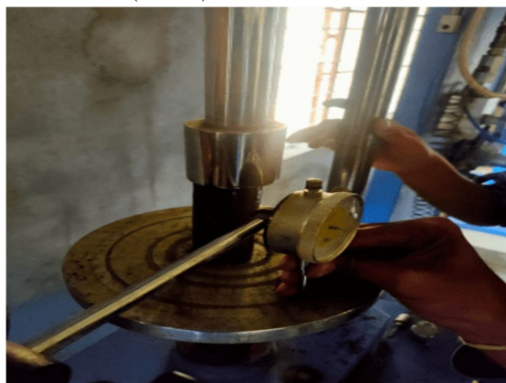
Fig.2. Normal Soil Specimen Undergoing UCS Test
