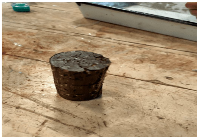
Figure 10 UCS specimen of Mix
