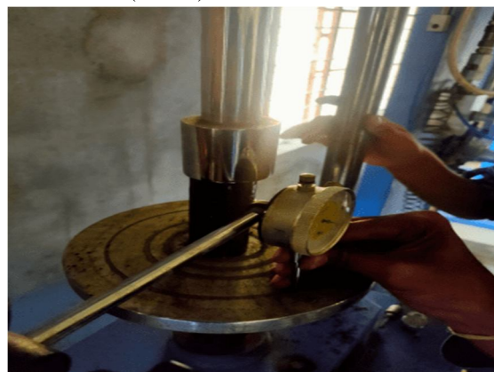
Fig.2. Normal Soil Specimen Undergoing UCS Test
