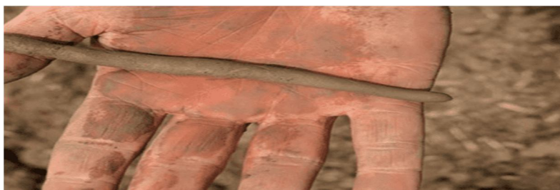
Fig.8 Plastic limit Soil Thread
