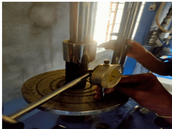
Fig.2. Normal Soil Specimen Undergoing UCS Test
