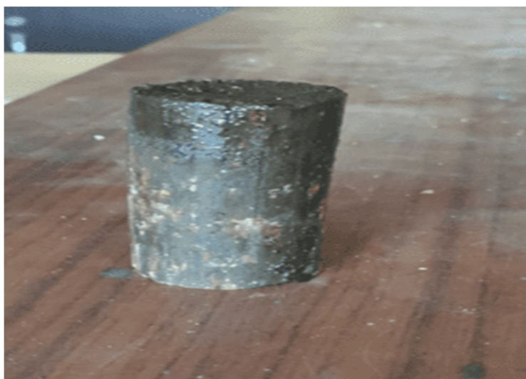
Figure 9 UCS specimen of Normal Soil
