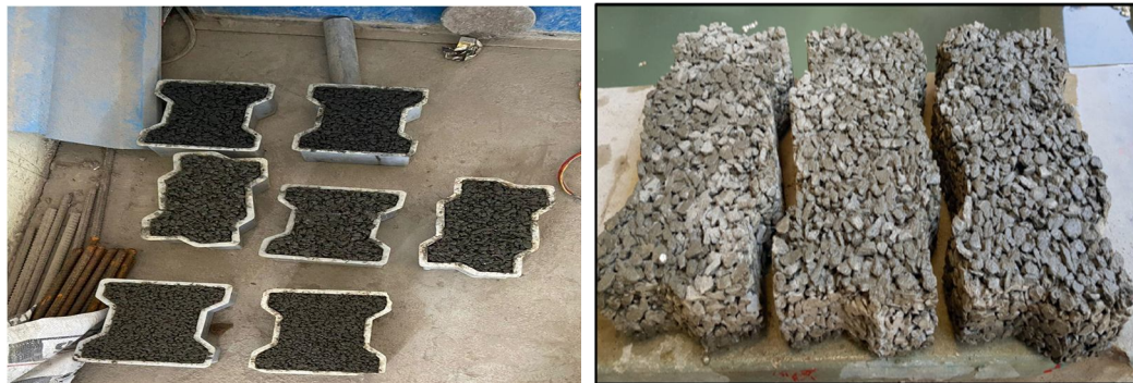
Figure 2: Preparation of paver block mould
