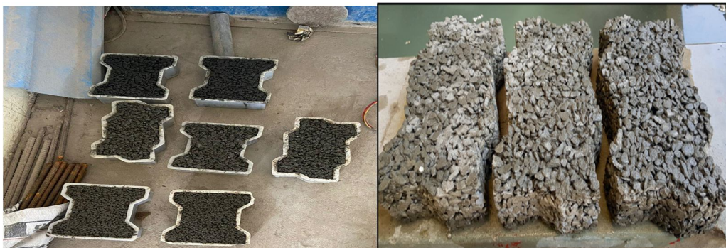
Figure 2: Preparation of paver block mould
