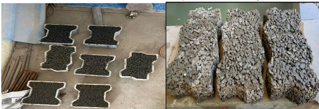
Figure 2: Preparation of paver block mould
