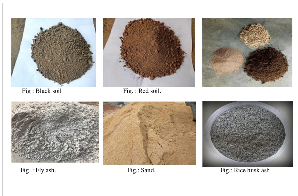
Fig.: Materials used for Rammed earth wall panel
