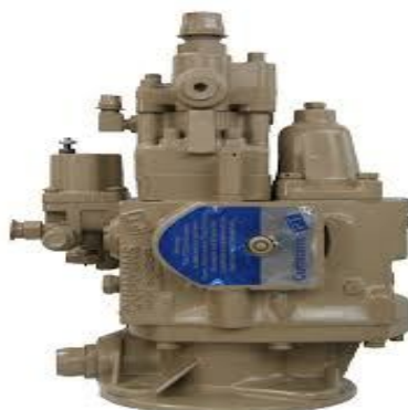
Figure-4 :Pressure Time Pump Assembly
