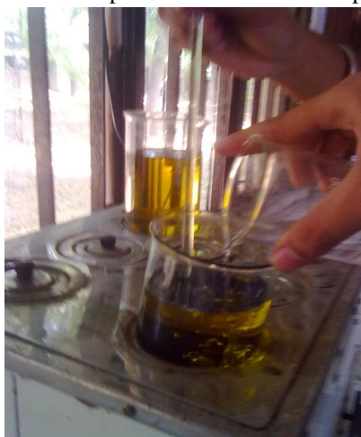
Figure 6: Stirring of Linseed oil and mixture of KOH & methanol at constant temperature 60°C
