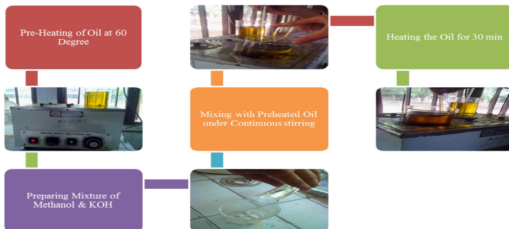
Figure 2: Process of Preparation of Methyl Esters (Biodiesel)
