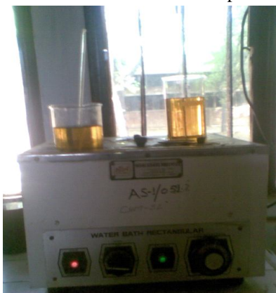
Figure 4: Pre-Heating Linseed raw oil on water-bath with stirrer
