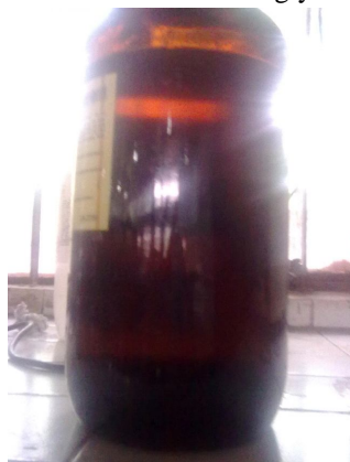
Figure 10: After 24 hours the glycerol sets down and methyl ester stay above
