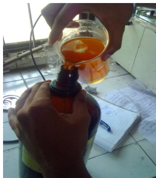
Figure 8: Pouring of mixture in separate container after stirring at constant temperature
