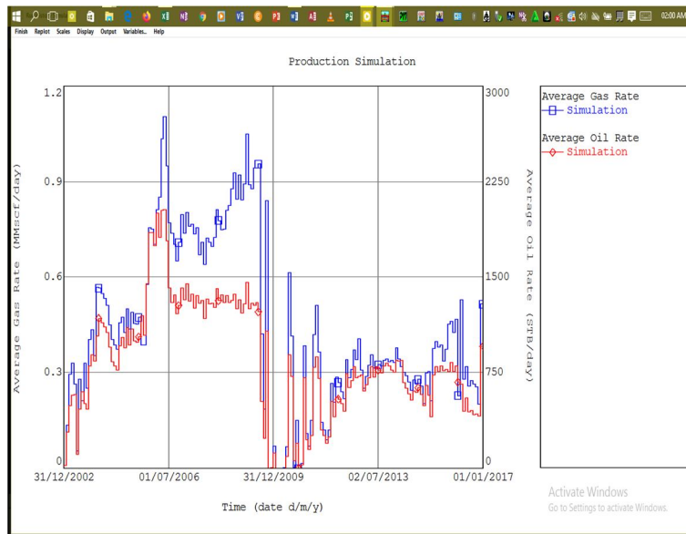
Figure 4.4 A comparison of the Stimulated Average Gas Rate (MMscf/day) and Stimulated Average Oil Rate (STB/day) against Time (date day/month/year)
