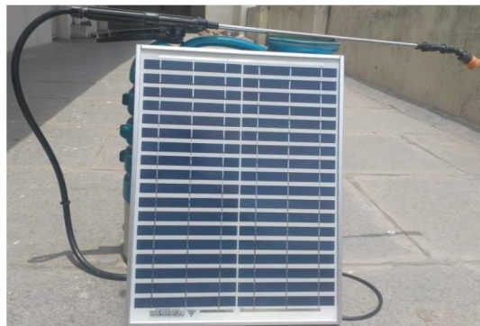
Fig.3 Fabricated solar pesticide sprayer (back sprayer)
