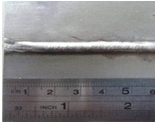
Figure 5: The samples of optimal welding condition.
