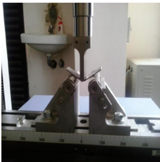
Fig 3. Specimen under bending test
