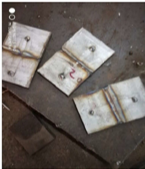
Fig 1(a). Butt Joint of SS310 and SS316 by TIG & MIG
