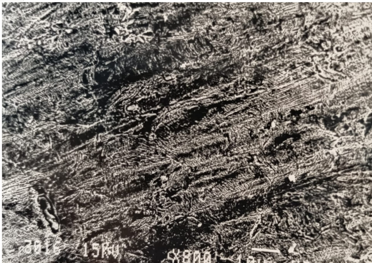
Fig. 3 SEM micrograph of mild steel surface exposed to 1.0M hydrochloric acid solution in presence of 400 ppm of DL-methionine for 12 hours (x 800).
