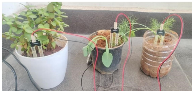
Fig 3.3 Three different Plants with soil moisture sensors
