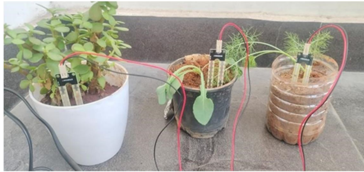
Fig 3.3 Three different Plants with soil moisture sensors
