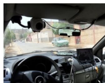
Figure 6 - Our system installed in the car based on IR camera
