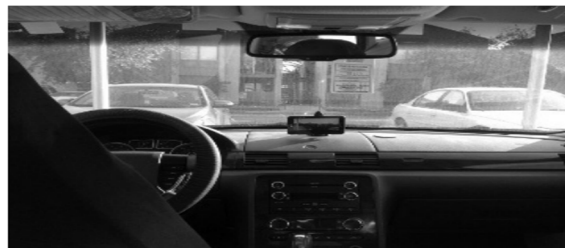
Figure 1 The system setup of the driver drowsiness detection using a smartphone.
