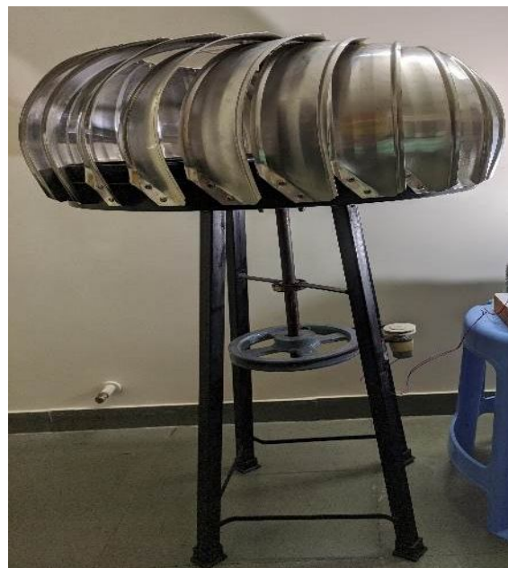
Fig. 2 Roof Ventilator with Pulley Arrangements
