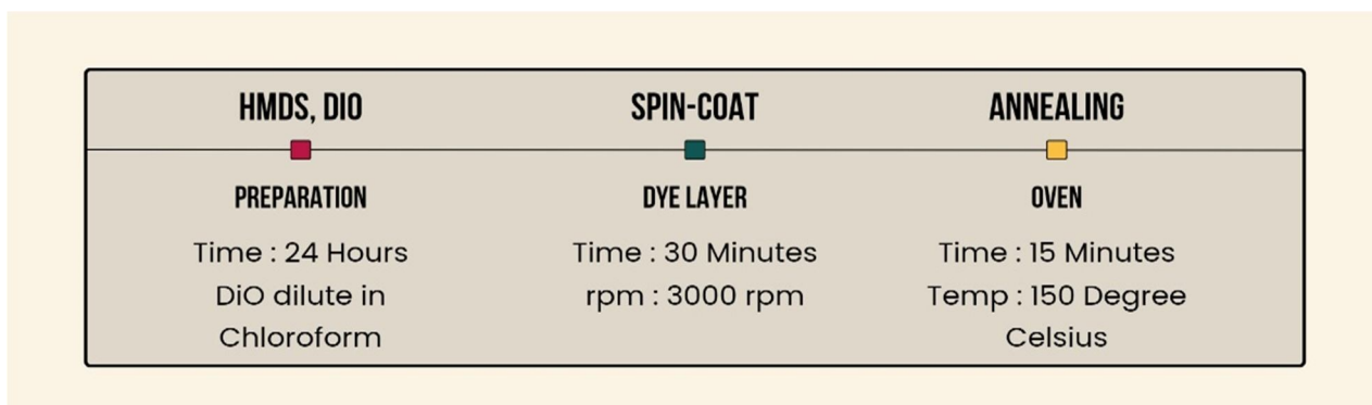
Figure 3 The process of dye deposition
