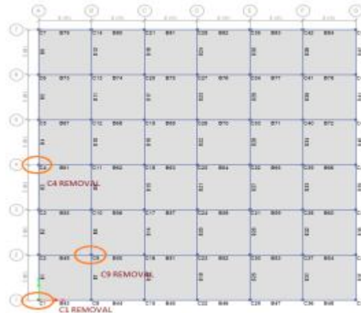
Fig. 2 3- Ready view of G+10 ETABS model with C-line removed
