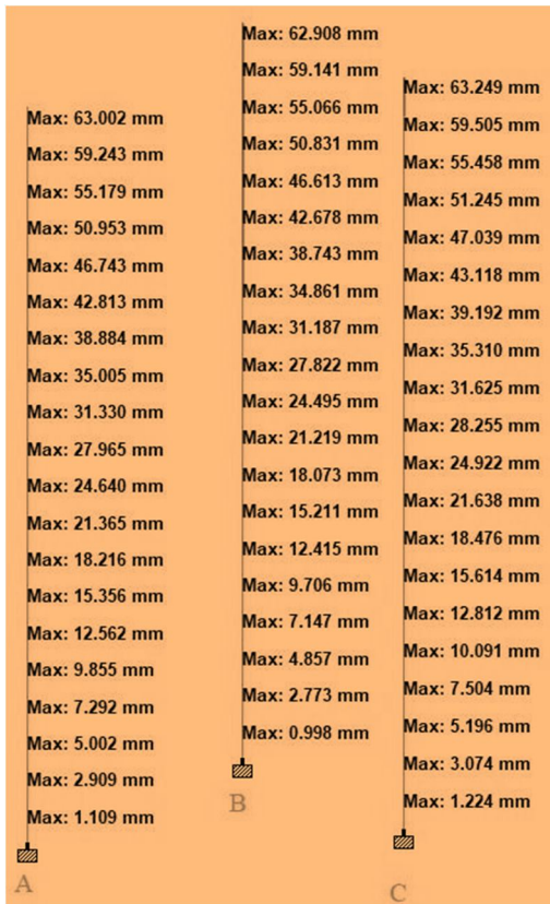
Figure 16. Displacement of Type E Building.
