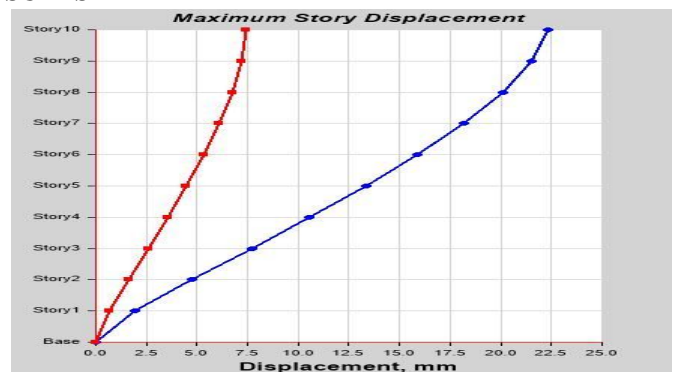
Fig. 5 Maximum storey Displacement (staircase is in corner)
