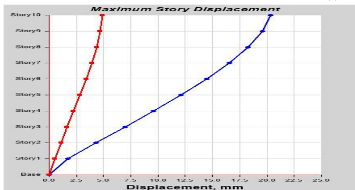
Fig. 4 Maximum Storey Displacement (staircase is in center)
