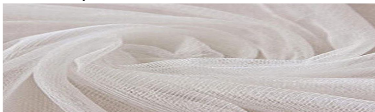
Fig 1. Net material used at innermost layer to curing pad
