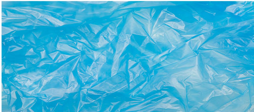
Fig.3. Plastic used in curing pad to prevent water from evaporation
