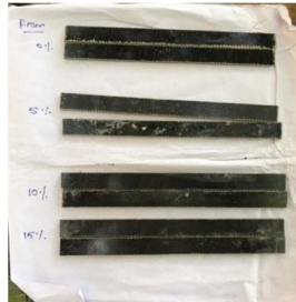
Figure1.6: Samples according to their filler percentage.
