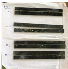
Figure1.6: Samples according to their filler percentage.
