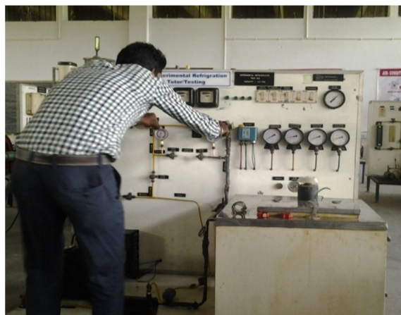
Fig.8:- Installation of Pressure Guages
