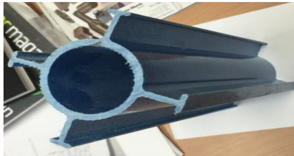
Fig. 1 Hollow Composite Reinforced Section (HCRS)
