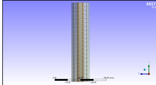
Fig. 4 Model of column with lateral hoops
