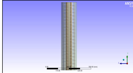
Fig. 4 Model of column with lateral hoops
