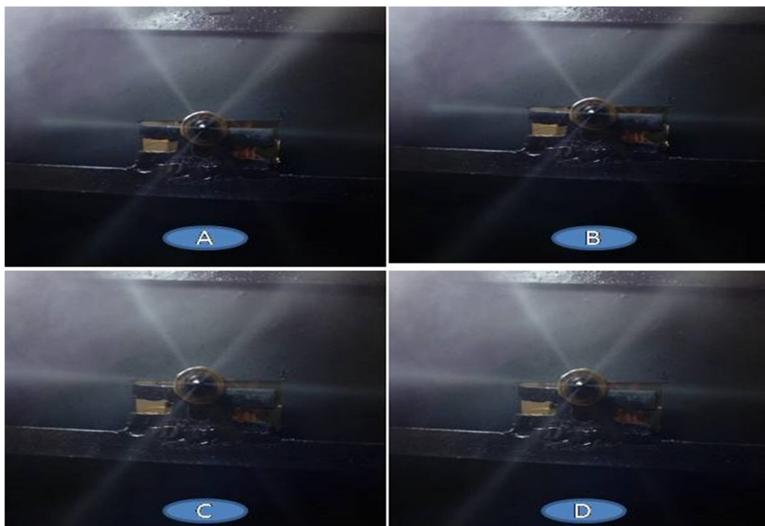
Figure 2 Fuel injection from 6-hole nozzle (A) at 20 MPa (B) at 30 MPa (C) at 40 MPa (D) at 50 MPa
