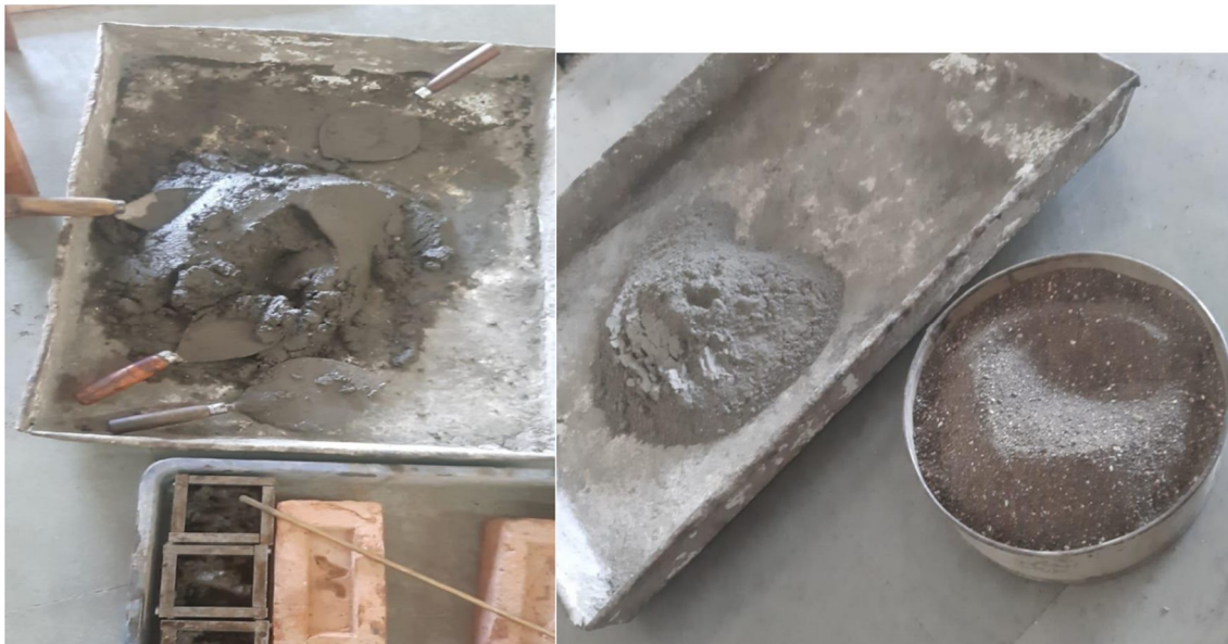
Fig.4 Mixing of Mortar
