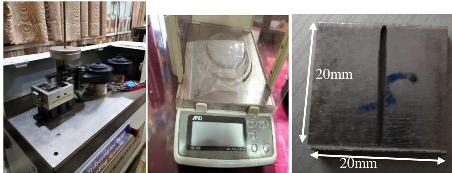
Fig 3 (a) Tribometer (b) weighing balance (c) specimen
