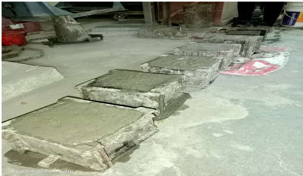
Fig. 4 Freshly prepared concrete blocks
