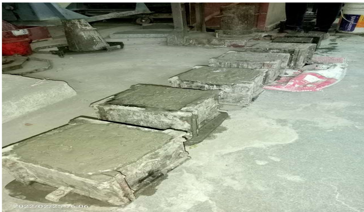
Fig. 4 Freshly prepared concrete blocks
