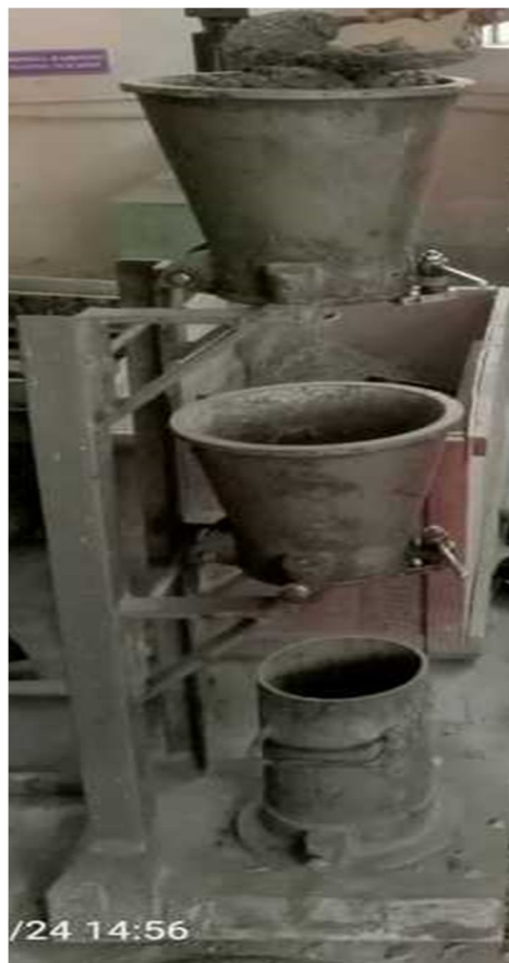
Fig. 3 Compaction factor test
