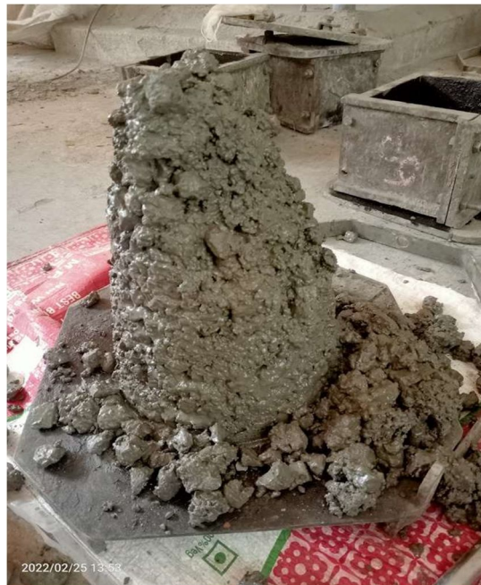
Fig. 2 Slump cone test
