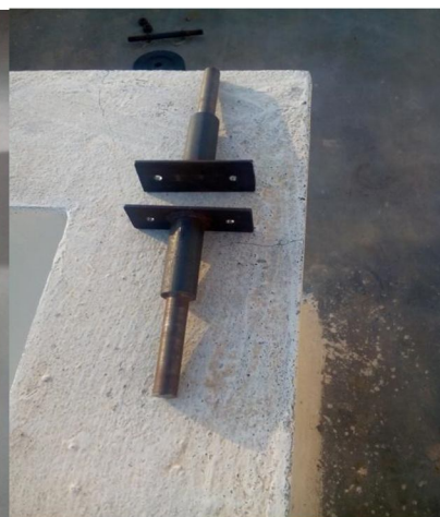
Fig. 3 Fixture for clamping of Cross lap joint in Universal Testing Machine
