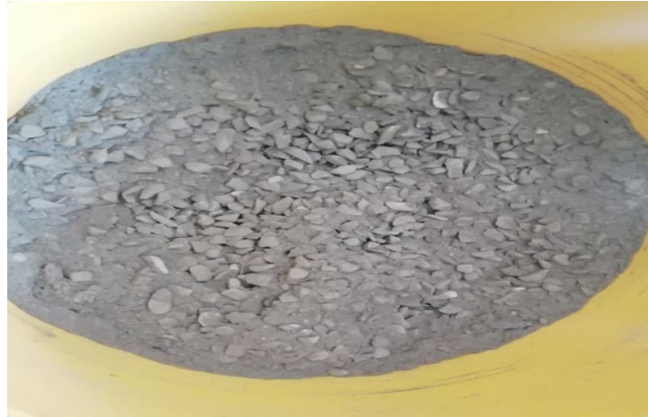
Fig. 3 Dry mix of concrete mix
