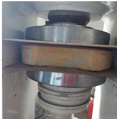
Fig. 7 Testing of sample in CTM
