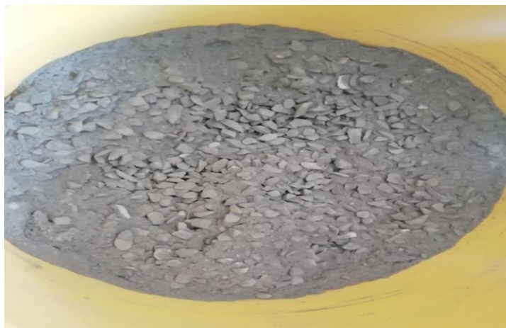
Fig. 3 Dry mix of concrete mix
