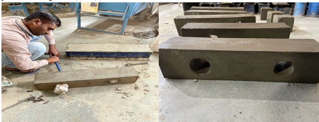
Fig. 4.4.4 (a) De-moulding of Beams
