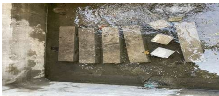
Fig. 4.4.4 (b) Curing of Specimens
