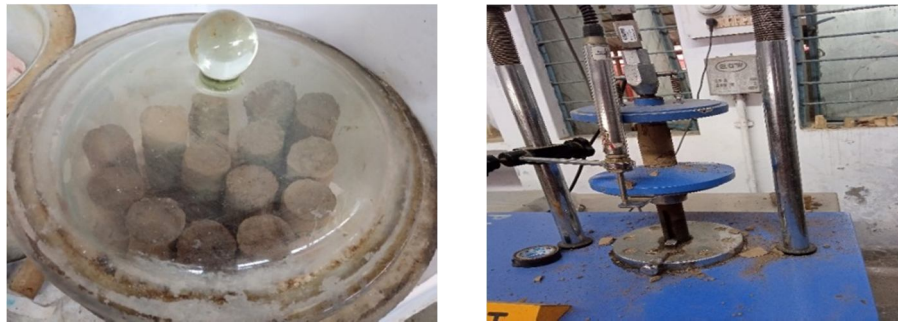
Fig. 3 UCS sample and test machine
