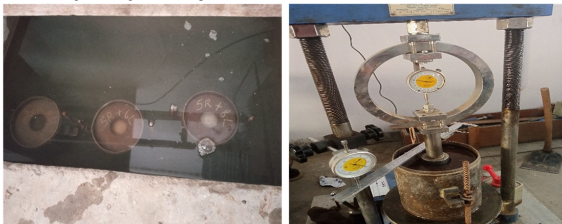
Fig. 4 CBR Soaked sample and CBR machine
