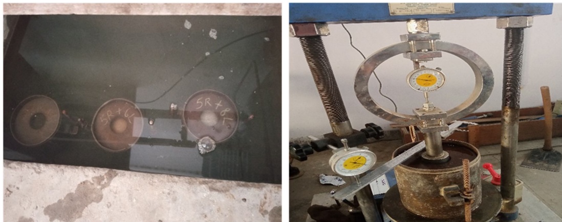
Fig. 4 CBR Soaked sample and CBR machine
