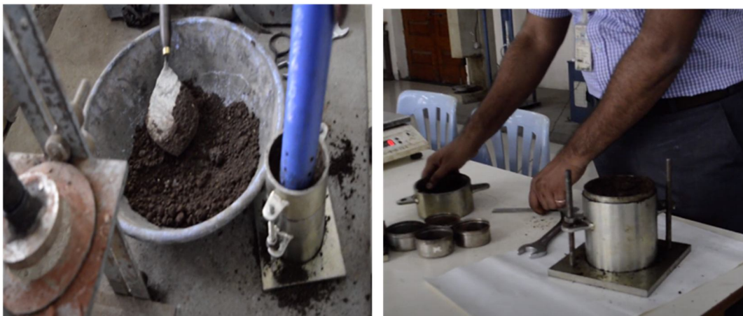
Fig. 3 Standard proctor test mould
