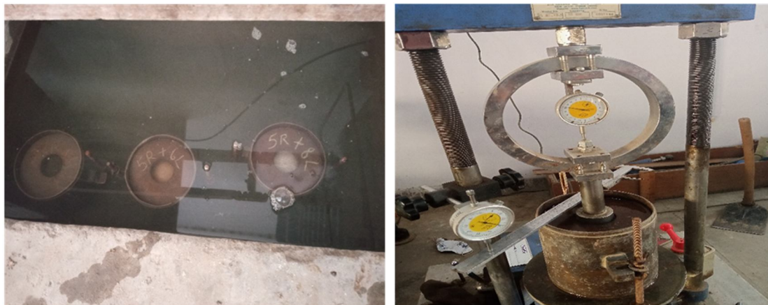
Fig. 4 CBR Soaked sample and CBR machine
