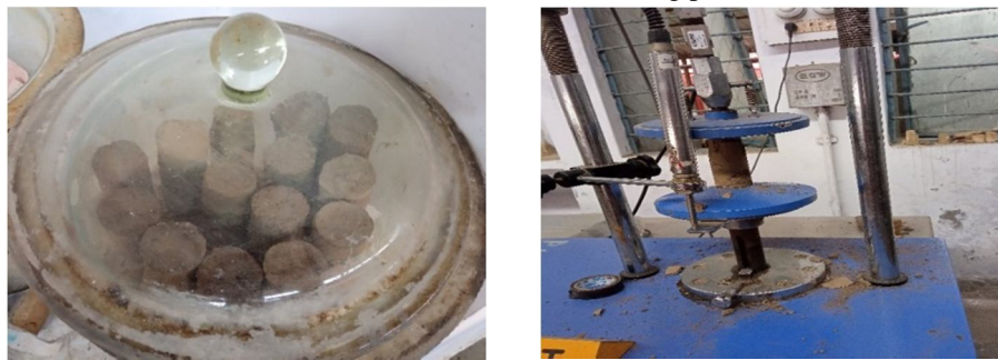
Fig. 3 UCS sample and test machine
