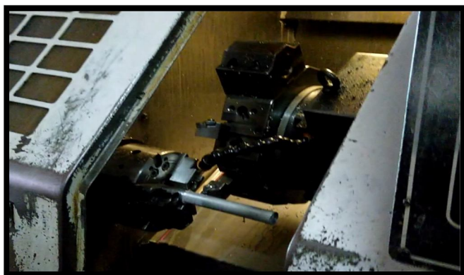
Fig.1.4 Machining of compression specimen
