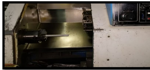
Fig.1.8. Machining of hardness test specimen
