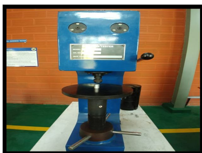
Fig.2.1 Brinell hardness testing setup
