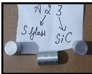
Fig.2.2 Specimen used for Brinell hardness test and formation of indent on specimen
