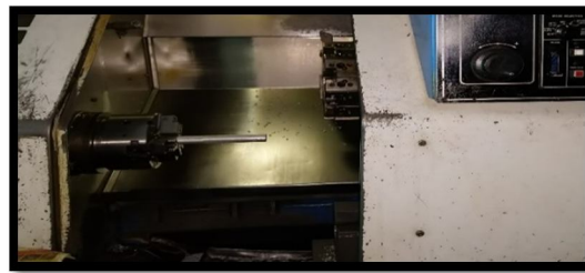
Fig.1.8. Machining of hardness test specimen
