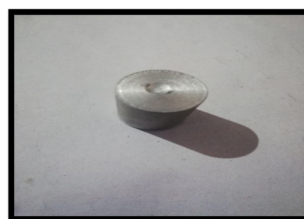
Fig.2.2 Specimen used for Brinell hardness test and formation of indent on specimen
