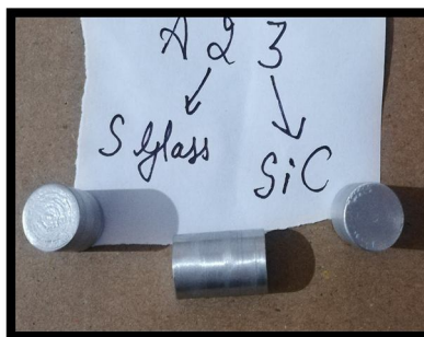
Fig.2.2 Specimen used for Brinell hardness test and formation of indent on specimen
