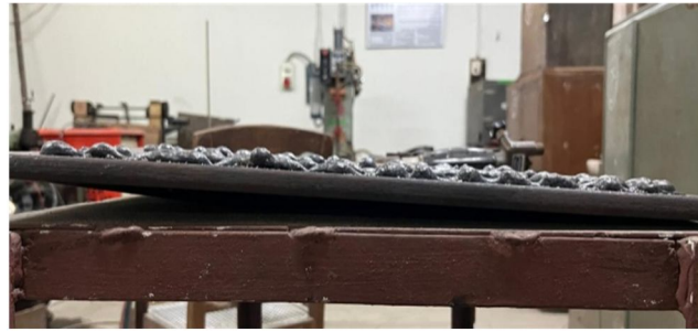
Fig.15 Non-Uniform Deposition Rate
