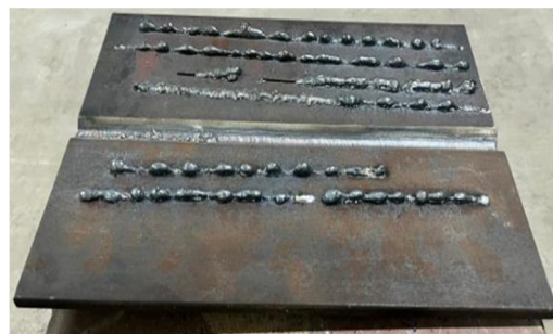
Fig.13 Bead on Groove - Side Angle View
