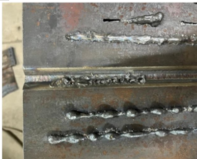
Fig.14 Bead on Groove - Top Angle View
