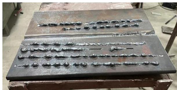
Fig.11 Bead on Plate - Side Angle View
