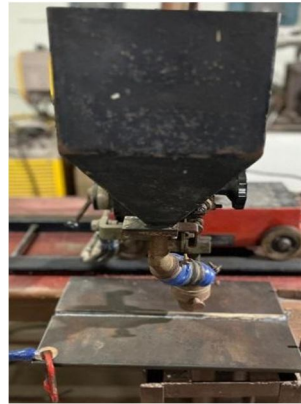
Fig.7 Welding Gun & Its Angle
