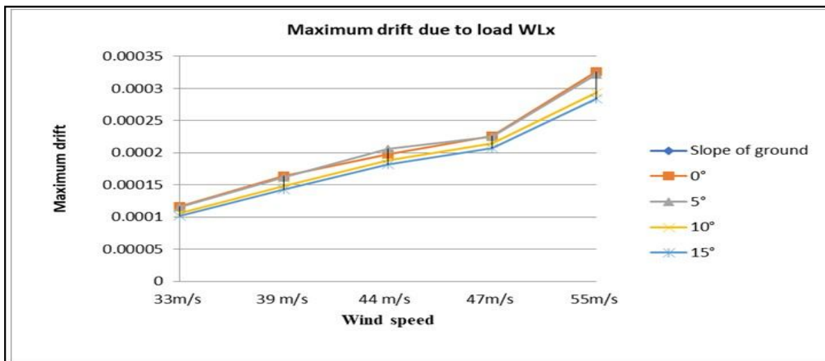
Maximum Displacement in 8 storey building frame due to load combination of 1.2(DL+LL+WL)
