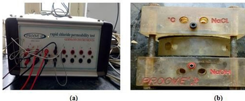
Fig 12: (a) PROOVE' it Microprocessor Power Supply Unit and (b) PROOVE' it Cell
