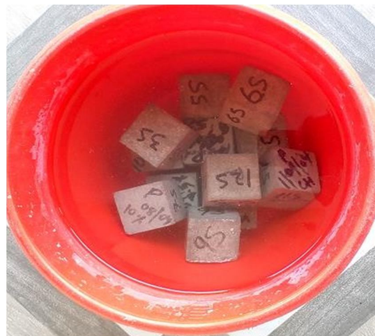
Fig 4: Immersion of Samples in 14% Solution of Sodium Sulphate Decahydrate
