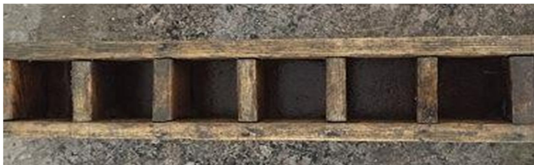
Fig 2: Moulds of Cubes of Size 50mm*50mm*50mm
