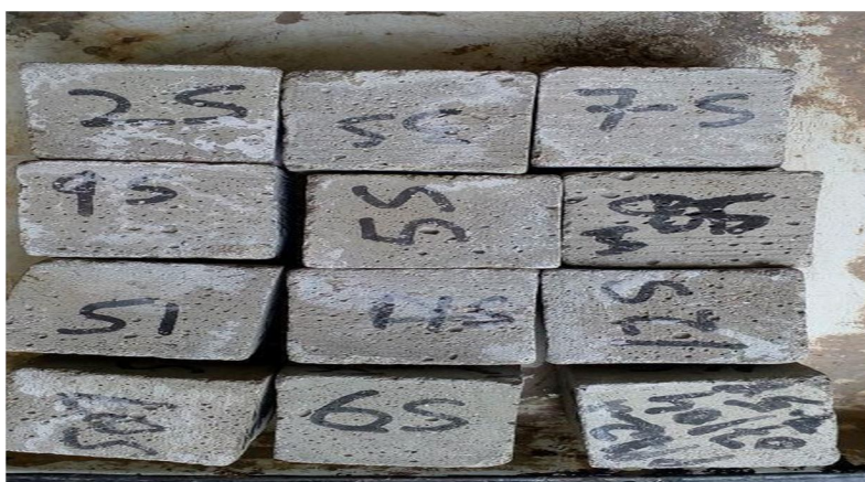
Fig 7: Physical Appearance of Mortar Treated with Sodium Sulphate solution
