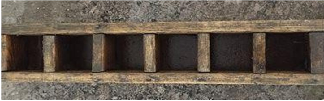
Fig 2: Moulds of Cubes of Size 50mm*50mm*50mm
