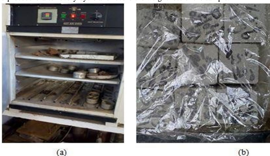
Fig 3: (a) Hot Air Oven and (b) Cubes Protected from Humid Atmosphere
