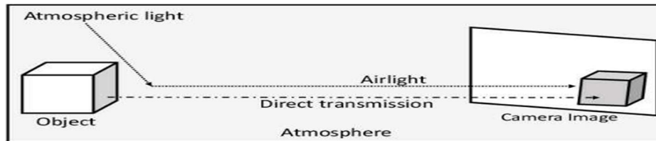
Fig.1 A Physical Picture of the day time haze imaging model [Yu Li, Robby T. Tan, Michael S. Brown]
