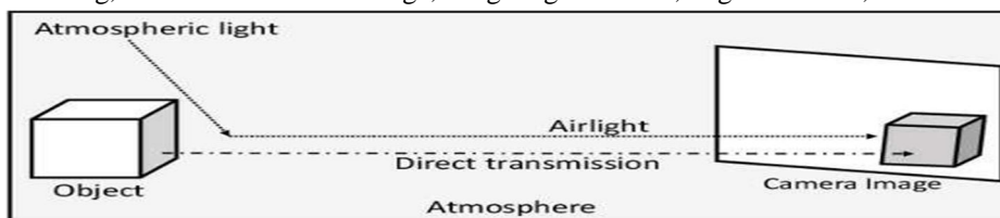
Fig.1 A Physical Picture of the day time haze imaging model [Yu Li, Robby T. Tan, Michael S. Brown]
