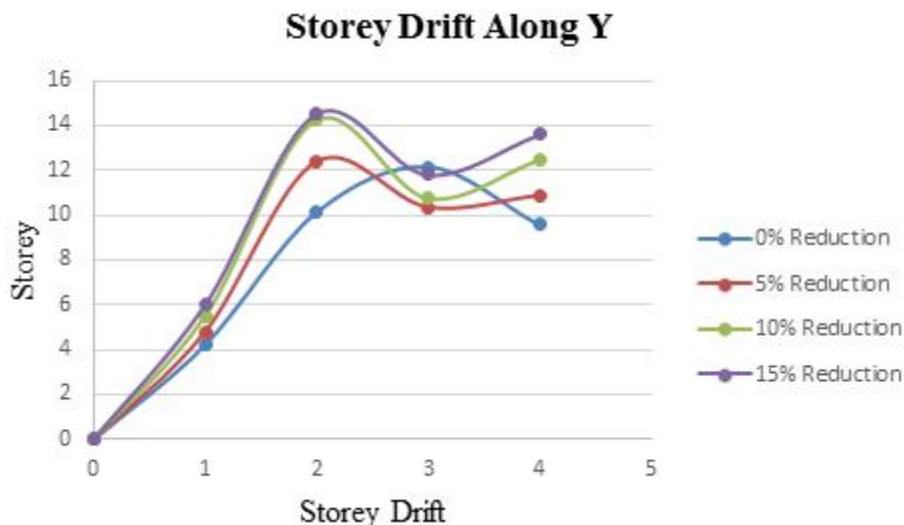
Fig. 7 Storey Drift of 0%, 5%, 10%, and 15% with 1.2 (DL + LL + EQY)
