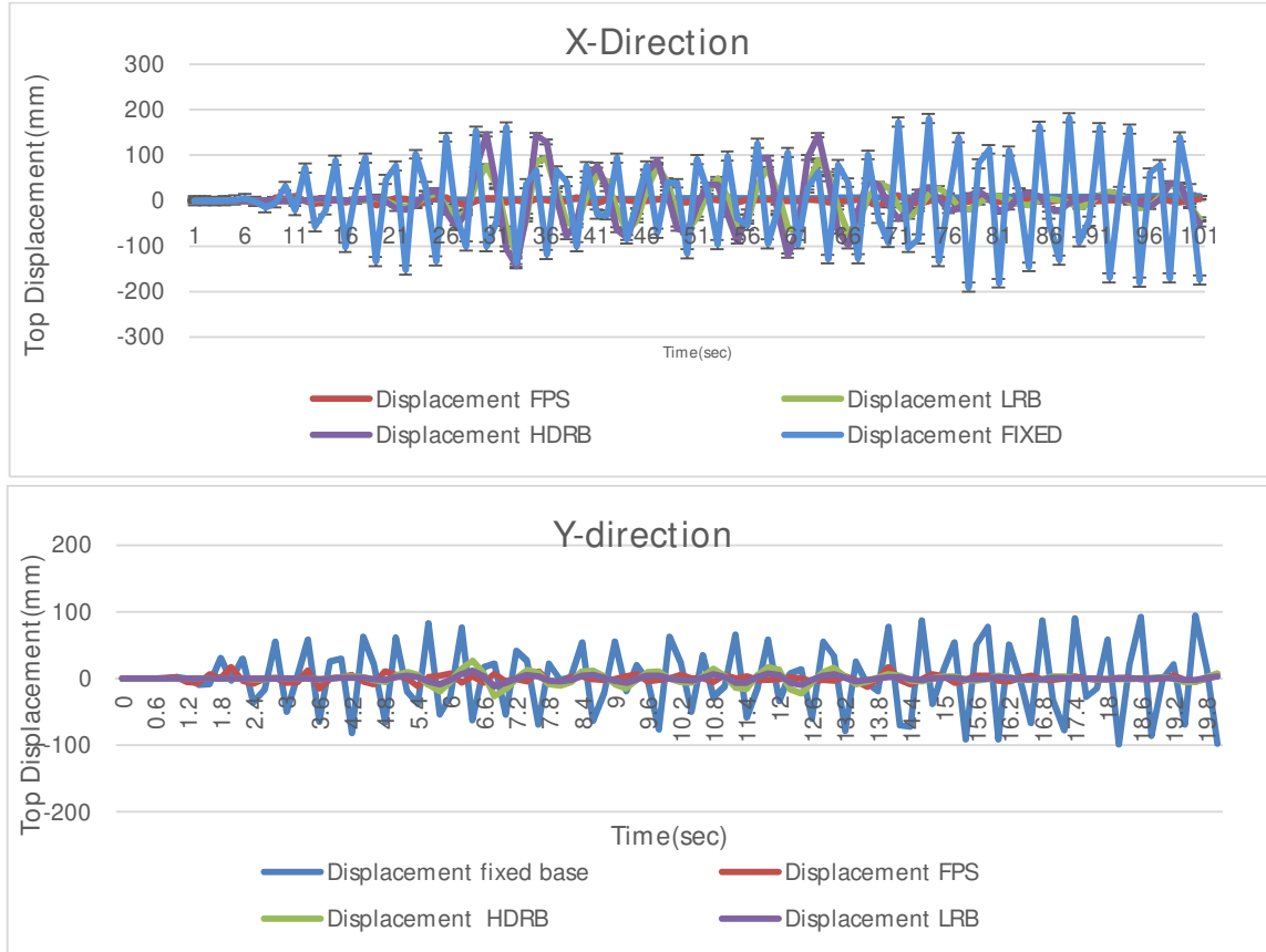
Fig. 5. Top displacement time history obtained for the base isolated (BI) model and fixed-base (FB) model under the NF earthquake from non-linear dynamic analysis.
