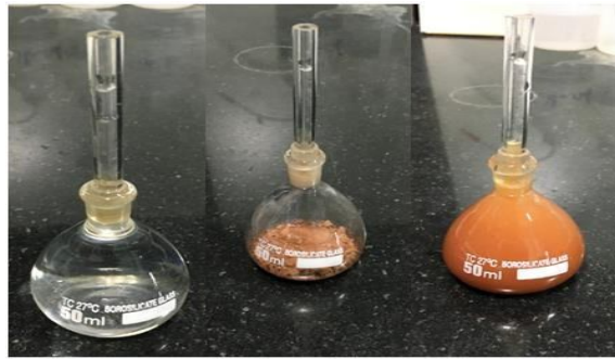
Figure 3.3 Specific gravity test by density bottle method
