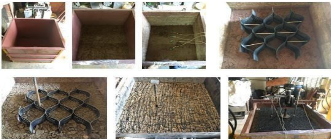
Figure 3.8 various stages for the preparation of the test section
