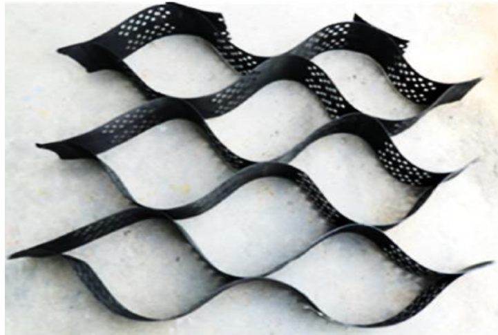
Figure 3.6 Typical geocell used in the study
