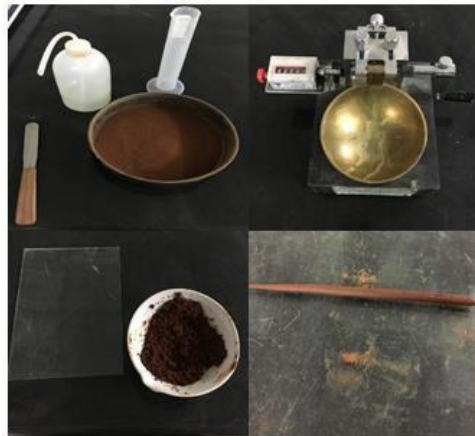
Figure 3.1 Images of the LL and PL test
