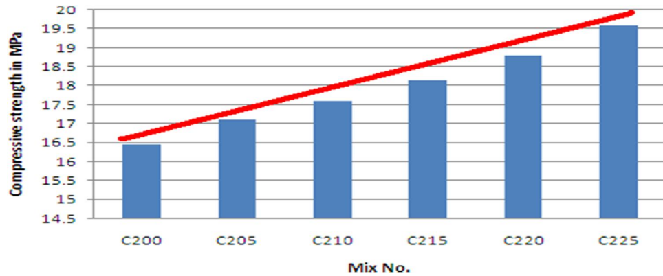
Fig. 9 – 14 days compressive strength of C2(Blended cement) category mix
