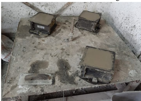
Cube Moulds filled with concrete
